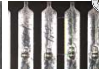
LED ring illumination (medium angles of incidence)
